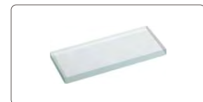
50mm reading scale (check magnification accuracy)
