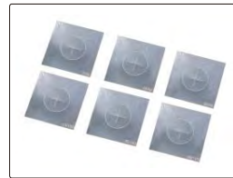
A1 standard sensitivity test piece (optional)
