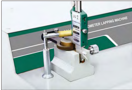
lapping measuring surfaces of caliper lower jaws
