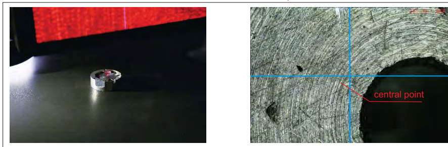
laser indicator locates the central point
